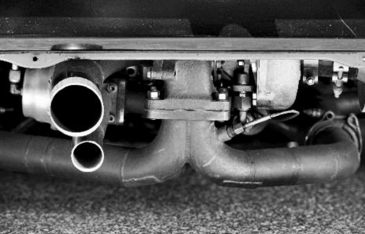
Wastegate is visible in this view of one of Deford's turbocharged 914s. Deford drives the car in PCA Club racing's GT3R category.
