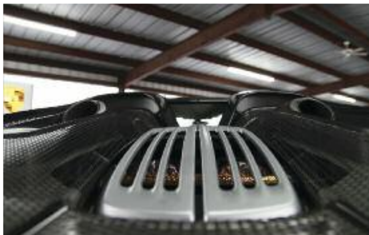
Above: The dual exhaust of the 918 roars from the top of the engine.
