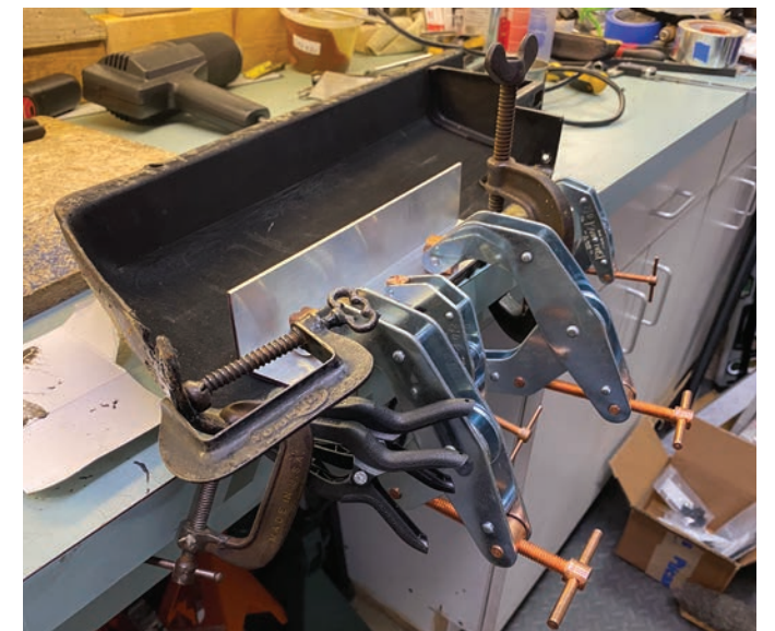
3) Reforming driver’s side pocket.
