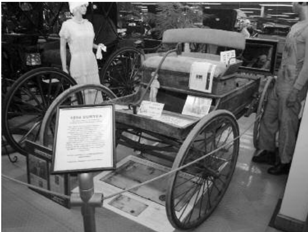
Above: Built in 1894, this significant automobile reshaped automobile production and innovation. This tiller-steered vehicle featured a differential rear end, disengaging hand crank and a three-speed bevel gear transmission. The car has original paintwork and on the underside of the floorboard was attached the original pencil drawing of the patented differential. Photo by Richard Curtis
