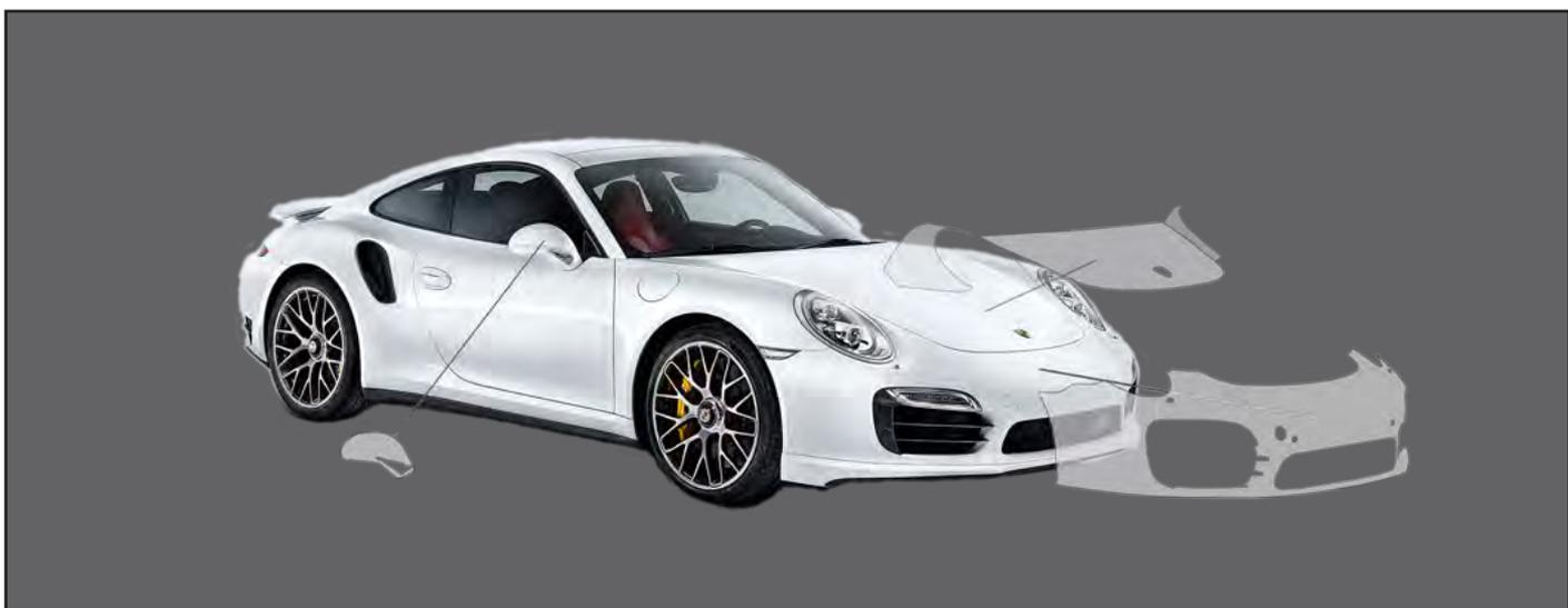
The typical Paint Protection Film (PPF) set protects the car from a frontal assault by debris
