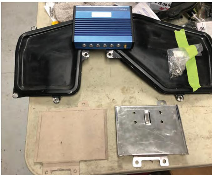
The CAD process at work, making a mounting bracket for the data collection system using a spare engine cover
