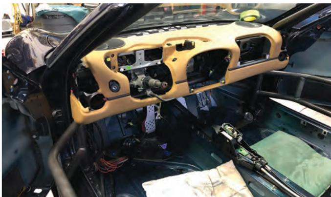
Dash fully fitted and installed
