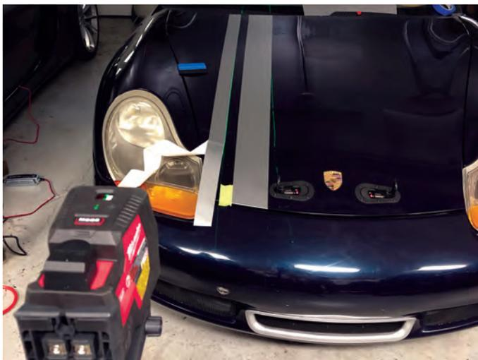
Using the laser level to ensure straight stripes
