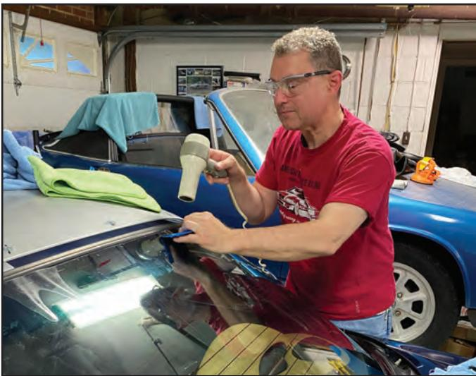
Finishing up installing the tear-offs
